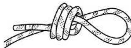
c) Scaffold knot with triple twist: loose
