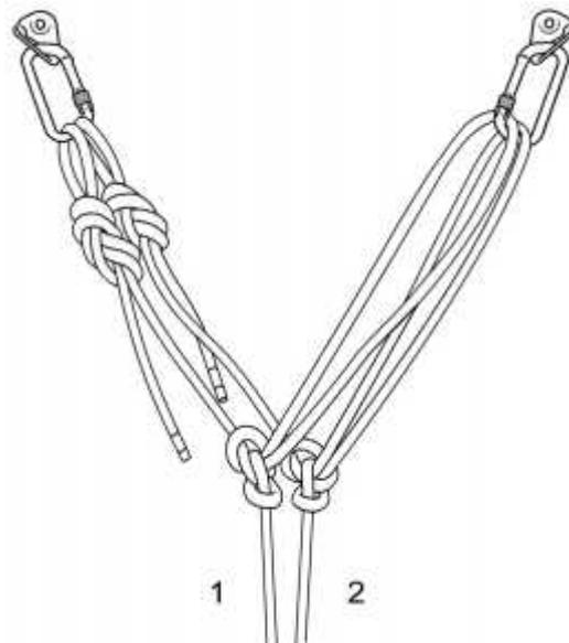
a) Example of a Y hang arrangement where the strength of each individual anchor is 15 kN or greater
