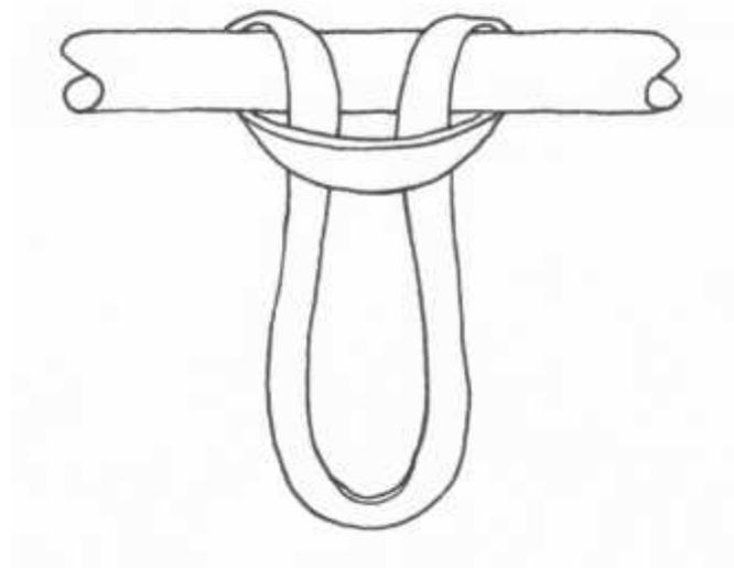
**Figure 2.7 — Example of a lark's-foot (choked) sling**
